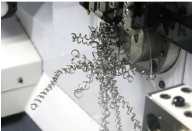
External coolant supply at normal pressure
